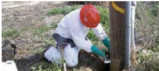
Pictured clockwise from top: Sundance Power Pole Inspectors logo, truck insignia and worker clothing; worker bores a hole for a sample of the wood; worker uses a hammer to test the soundness of the pole.
