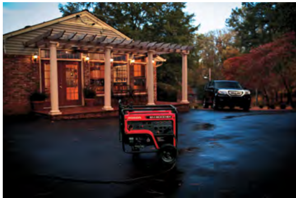
Position portable generators at least 25 feet outside the home, away from doors, windows and vents that can allow CO to enter the home. Photo Source: Honda
