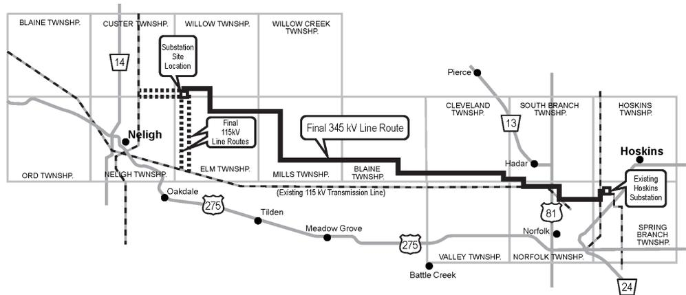
The line will be built several miles north of and generally parallel to U.S. Highway 275. When completed, the 345,000-volt line will run between a substation located on the northeast edge of Norfolk next to Nucor Steel and a substation northeast of Neligh. The 115,000-volt lines will connect the Neligh substation to other transmission lines.
